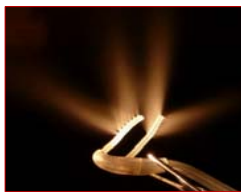
Figure 1: Photograph demonstrating the perfluorocarbon-oxygen spray in dorsal and lateral direction from the distal end of the nasopharyngeal paired tubing.
